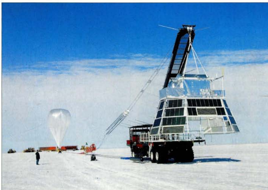
Balloon inflation prior to launching of the BESS-Polar spectrometer. The detector, with its solar-power cells, is in the foreground. The balloon reached an altitude of 37–39 km.
