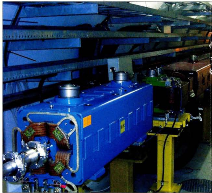
Installed section of TI 8 consisting of a main quadrupole (blue), followed by dipoles, all built by the Budker Institute for Nuclear Physics (BINP) in Novosibirsk.
