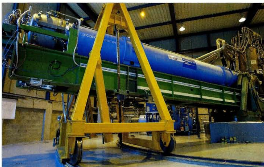
The CAST axion helioscope points towards the Sun each day at sunrise and sunset.
