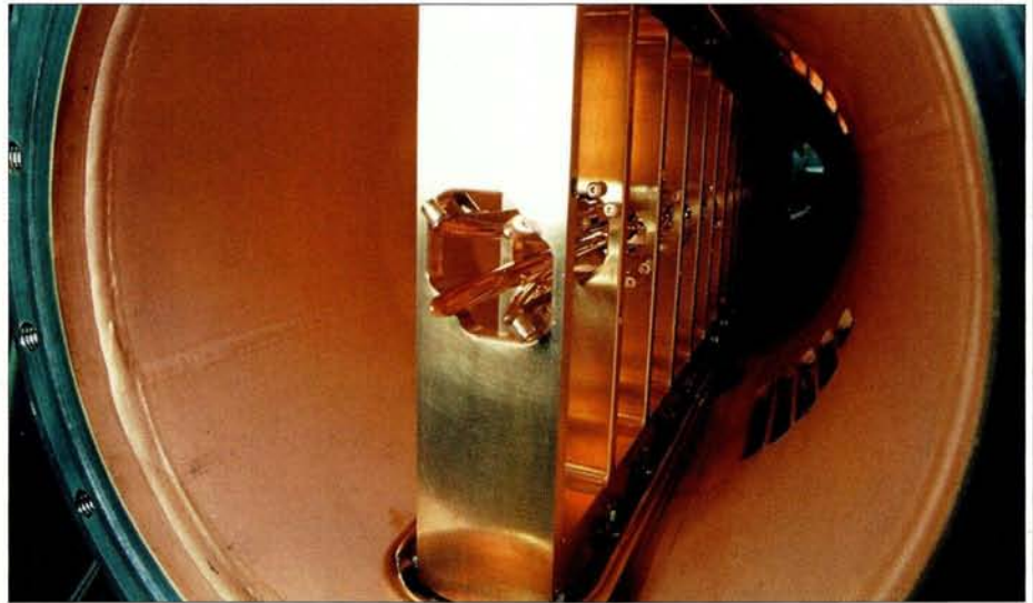
ASACUSA's radio-frequency quadrupole decelerator, open to show the four-rod structure along the centre, which crosses 35 resonator chambers formed by the vertical partitions.
